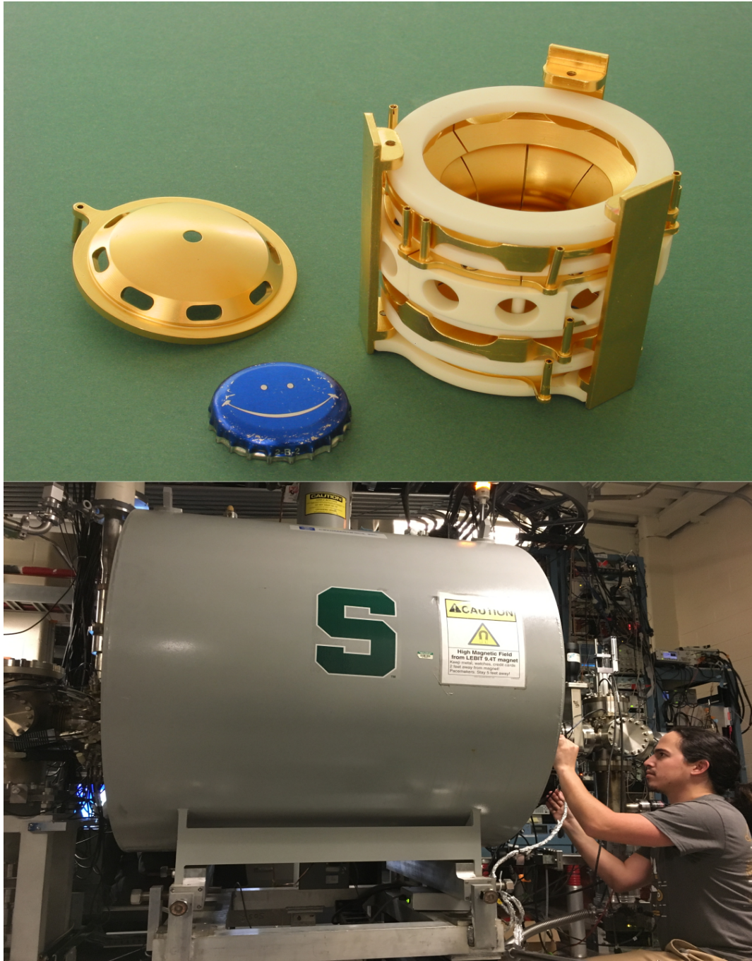
Figure 2.7: The Penning trap used at the LEBIT facility to perform high-precision cyclotron frequency measurements of rare isotopes. The Penning trap is housed in the 9.4 T superconducting solenoid magnet.
