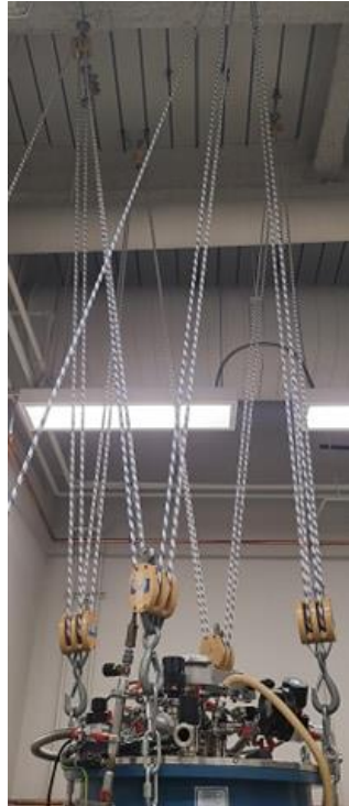
Figure 2.7: The entire cryostat, microscope included, can be suspended off the floor by bungee cables, decoupling the cryostat from low frequency building vibrations.
