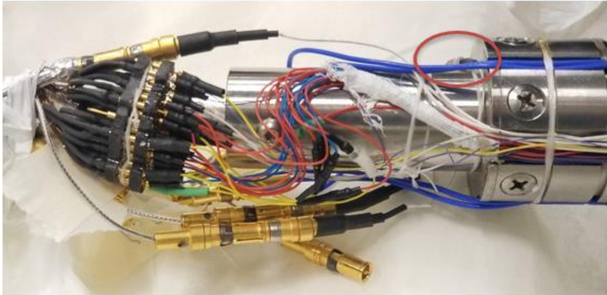
Figure 2.10: Image of the connections above the functional scan head during a rebuild. The blue wires are the four electrical leads used to connect the SCQDM. The large connections are the bias voltages supplied through each of the walking piezo tubes. The smaller connections in black are generally connected to the outside of the piezo tube and are responsible for sending the walking waveform to the appropriate quadrant. Lastly, circled in red is the Allen Bradley resistor, which sits just above the scan head and tracks the temperature of the microscope during push downs.
