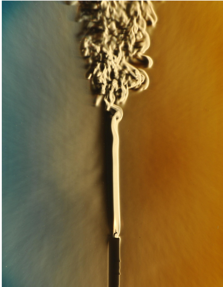
Figure 1.4: Schlieren photograph showing the thermal plume of a lit candle, showing the smooth rising flow starting from the base of the flame that transitions into turbulence at the top of the flame. As a gas, the viscosity in smoke and air is low; thus, the velocity of the uplifted heated gas is sufficient to create a high Reynolds number flow, with Re \gtrsim 10^3 , which is prone to fluid instabilities. The laminar flow originating from the flame decays into turbulence as these instabilities grow further down the flow.
