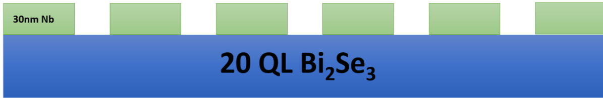
Figure 6.8 The completed device after removing the remaining e-beam resist.
