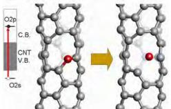
Fig. 3: Photo-induced de-oxidation of a defective carbon nanotube.
